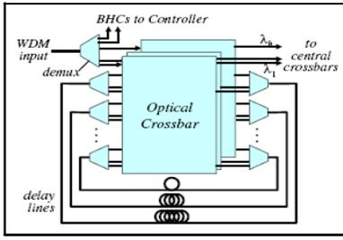
Figure 1: 1, 2, ..., N-1 OTSI Architecture
